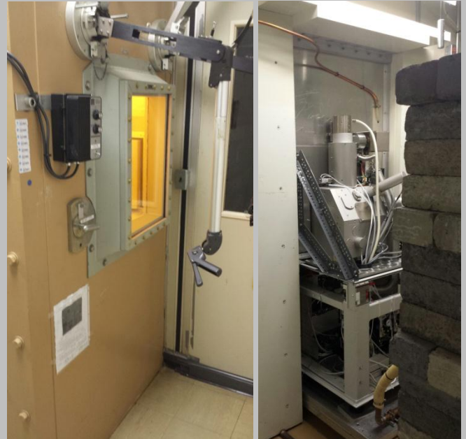
MCOE SEM hot cell viewing window with manipulator (left) and 2012 Tescan Vega3 XMU SEM (right)
