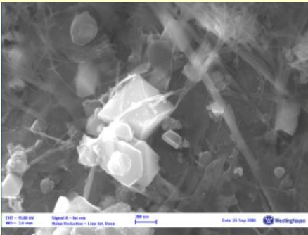
Oxide deposits on the ID surface of an Alloy 600 steam generator tube
