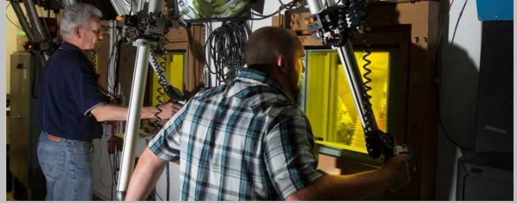
MCOE radiological technicians operating hot cell manipulators
