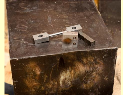
Machining of surveillance capsule test specimens from archive material ingot
