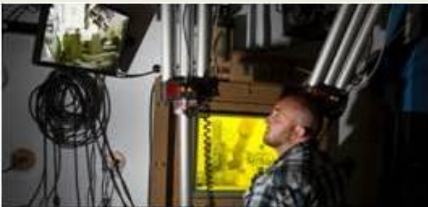
MCOE radiological technician performing work in the high level hot cell using remote cameras and live video feed monitors
