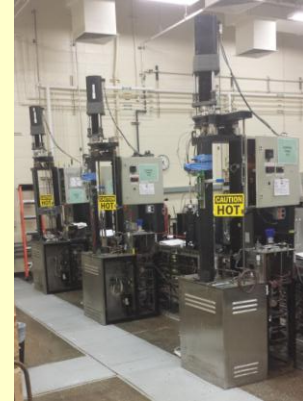
Autoclaves equipped with load frames
