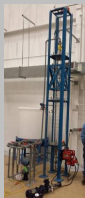
Design and Fabrication of the 4" Intermediate Loop
