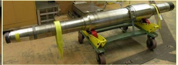
Cracked reactor coolant pump shaft
