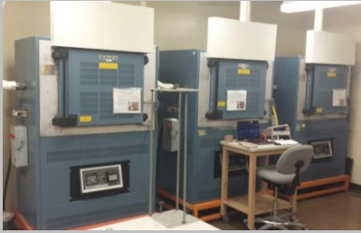
3-M Blue Box air furnaces
