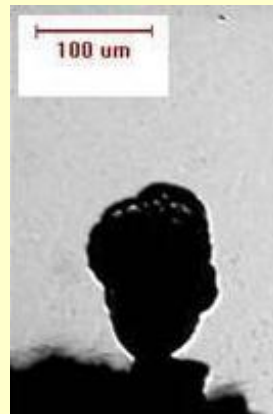
Pitting from microbial attack
