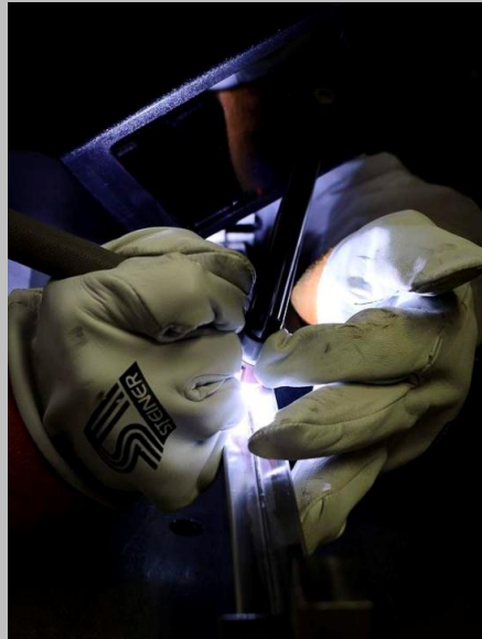
GTAW of a surveillance capsule
