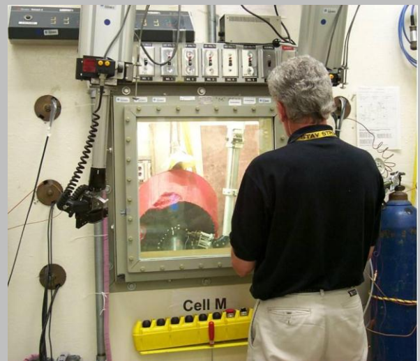
Eddy current examination in low level hot cell of approximately 800 pound section with full penetration flame cut from retired reactor pressure vessel head
