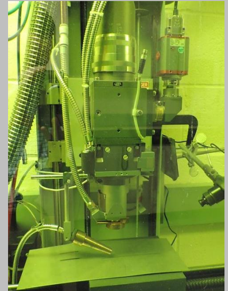
Nd:YAG laser welding head with video feedback system, air knife, and multi-axis positioning
